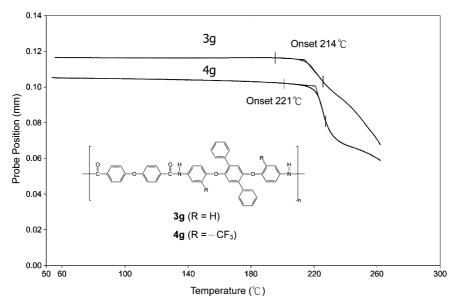
Fig. 3. TMA thermograms of polyamides 3g and 4g at a heating rate of 10 °C/min.
