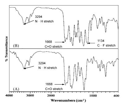
Fig. 1. (A) The FTIR spectrum of polyamide 3b and (B) the FTIR spectrum of polyamide 4b.
