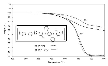
Fig. 4. TGA curves of polyamides 3d and 4d at a heating rate of 20 °C/min.
